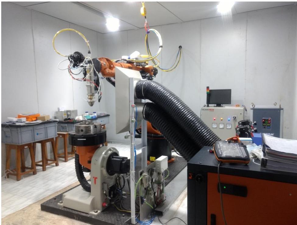
Laser materials processing (6 kW, GaAs Laser) facility has been developed under the project (as a Co-PI, PI: Prof. I. Manna) sponsored by Department of Science and Technology, N. Delhi and installed in the Steel Technology Center.
