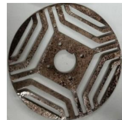
Fig: Fabricated prototype of Synchronous Reluctance Motor (3 kW peak power, 17.5 Nm peak Torque)
