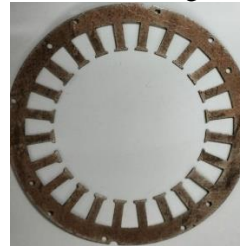
Fig: Fabricated prototype of Synchronous Reluctance Motor (3 kW peak power, 17.5 Nm peak Torque)
