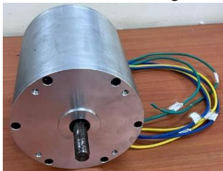
Fig: Fabricated prototype of Synchronous Reluctance Motor (3 kW peak power, 17.5 Nm peak Torque)
