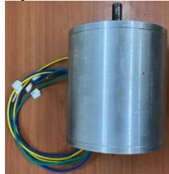
Fig: Fabricated prototype of Synchronous Reluctance Motor (3 kW peak power, 17.5 Nm peak Torque)
